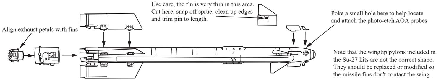
Some material may need to be removed from the mounting brackets to allow the missiles to fit the pylons included in your kit.
